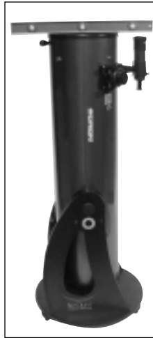
Figure 8. Once the base is leveled, point the tube up until the mirror cell comes into contact with the vertical stop. Then, place the carpenter's level across the top of the tube as shown. If the vertical stop is set properly, the top of the tube should also be level.
