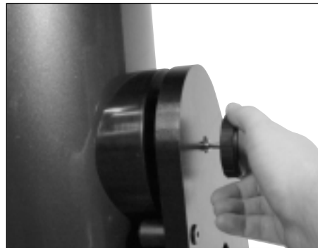
Figure 6. The retaining knob now goes through the shaft of the altitude encoder assembly before threading into the side bearing on the telescope tube.
