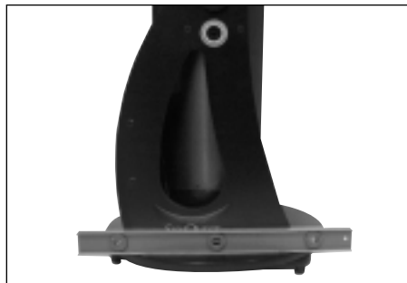
Figure 7. Place a carpenter's level on the base as shown. The base should stay level through a 180° rotation in azimuth. Once the vertical stop is set, the base does not need to be level to function properly.
