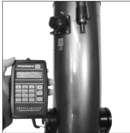
Figure 9. If you stand to the left of the telescope, and face the direction the tube is pointing, the guide arrows will correspond exactly with the direction you should move the telescope in order to find the selected object.
