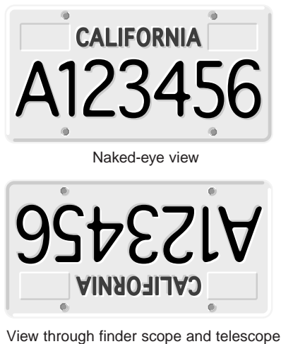
Figure 11. The view through a standard finder scope and reflector telescope is upside down. This is true for the SkyQuest and its finder scope as well.
