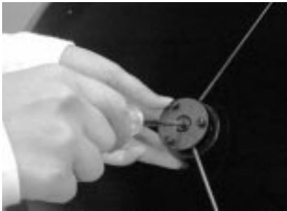
Figure 15. To center the secondary mirror under the focuser, hold the secondary mirror holder in place with your fingers while adjusting the center screw with a Phillips screwdriver. Do not touch the mirror's surface!
