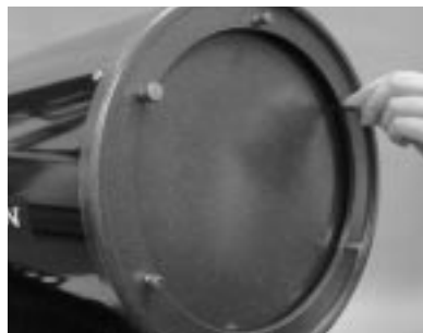
Figure 18: The tilt of the primary mirror is adjusted by turning one or more of the three spring-loaded collimation thumb screws.
