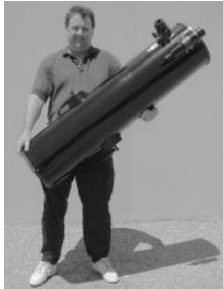
Figure 12: You can carry the tube by grasping the tube with one hand while grasping the mirror cell end with the other.
